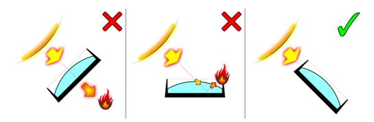
Figure 1. Avoiding damage from light sources
