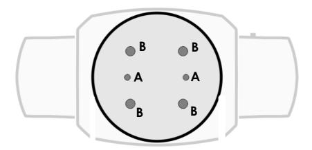
Figure 8 Mounting points in base
