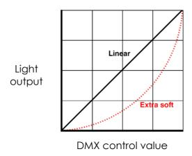
Figure 7. Dimming curves
